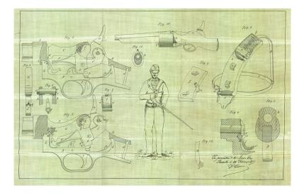
In addition to the rifle-action patent drawings, Lee designed some snazzy accessories, including a spring-loaded over-the-shoulder-box that would deposit a fresh cartridge at the opening—a box magazine, just not one mounted to the rifle...Yet!
