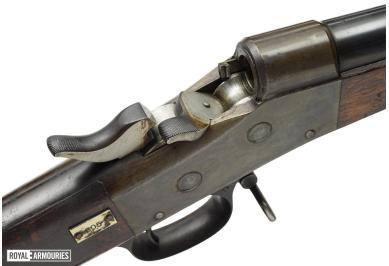
*Source:* The Royal Armouries—National Firearms Ctr. Leeds, UK. The wonderfully simple breech loading action of the Remington rolling block. The hammer is cocked, the breech rolled back to expose the chamber, simultaneously forcing the extractor back, a new cartridge is inserted into the breech, and the chamber rolled forward to close. On firing, the articulated block that mounts the hammer under-rides the breech block, locking the action.
